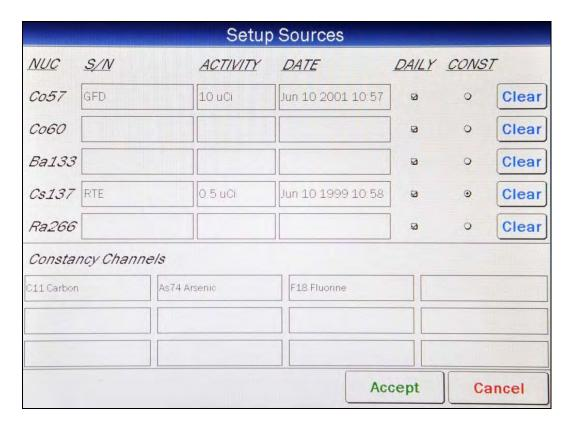
Figure 6-11 Setup Sources Screen
