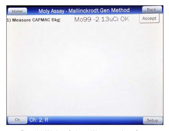
Figure 10-8 Moly Assay Background Measurement Accept Screen
