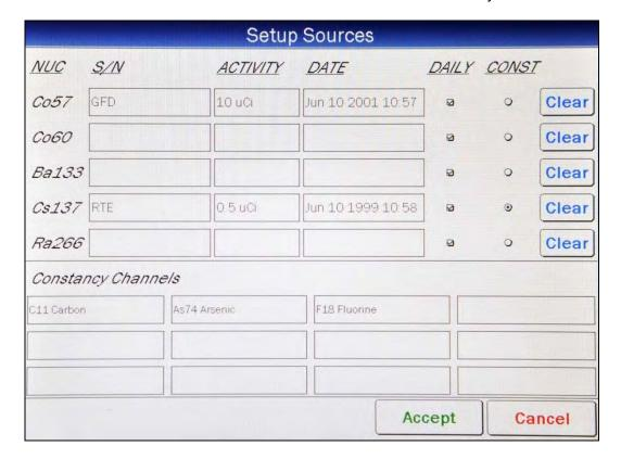
Figure 6-15 Setup Sources Screen
