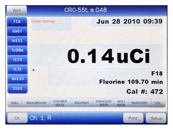
Figure 8-1 Chamber Measurement Screen
